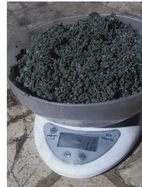
Gambar 4.8 hasil residu pirolisis mie instan 1000 gram
