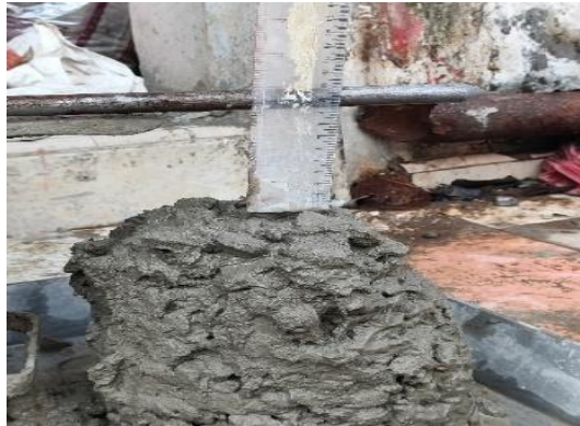
Figure 1. Slump Test Source: Primary data, 2024
