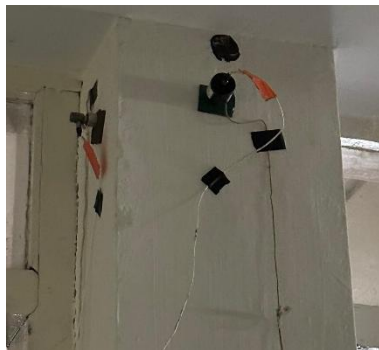
a. Position of the sensor on the ring beam
