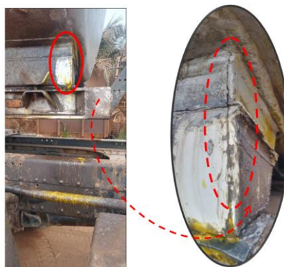
Figure 5. Leakage on the Bottom Side of the Front of the Tank
