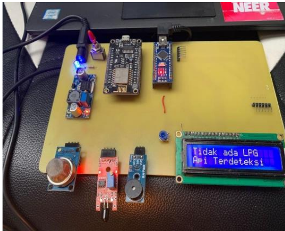
Figure 5. Equipment testing when a fire is detected and LPG is not detected
