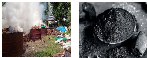
Figure 4. Coconut Shell Ash before and after combustion
